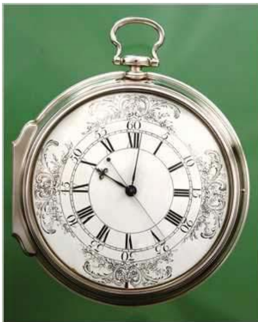
Figure 7.3 John Harrison's fourth marine chronometer from 1760. By courtesy of the National Maritime Museum
