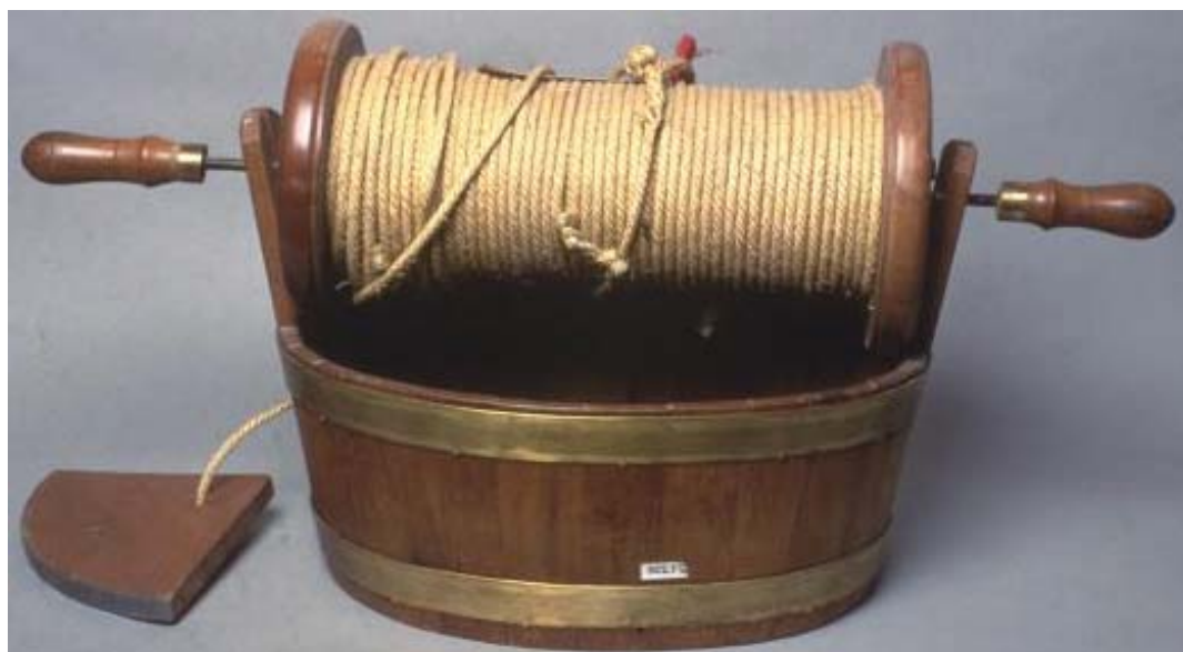
Figure 1.2 A typical logship, logline and reel used to measure a ship's speed. By courtesy of Archivo del Museo Naval, Madrid
