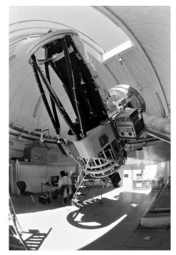
Fig. 1. Multichannel photopolarimeter used for measuring the sky polarization was mounted behind the 1 m Jacobus Kapteyn Telescope at La Palma. As the primary objective of our campaign required daytime observations of Venus down to a Sun separation of 13°, we mounted baffles and screens on the east side of the telescope to shield its primary mirror from direct and singly reflected sunlight [3–5].
